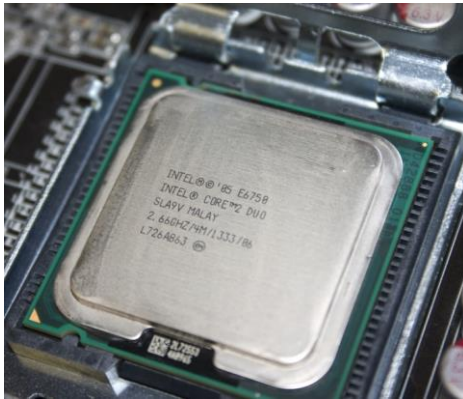
intel core duo (has 2 cores, 2.66 GHz)
