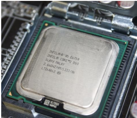
intel core duo (has 2 cores, 2.66 GHz)
